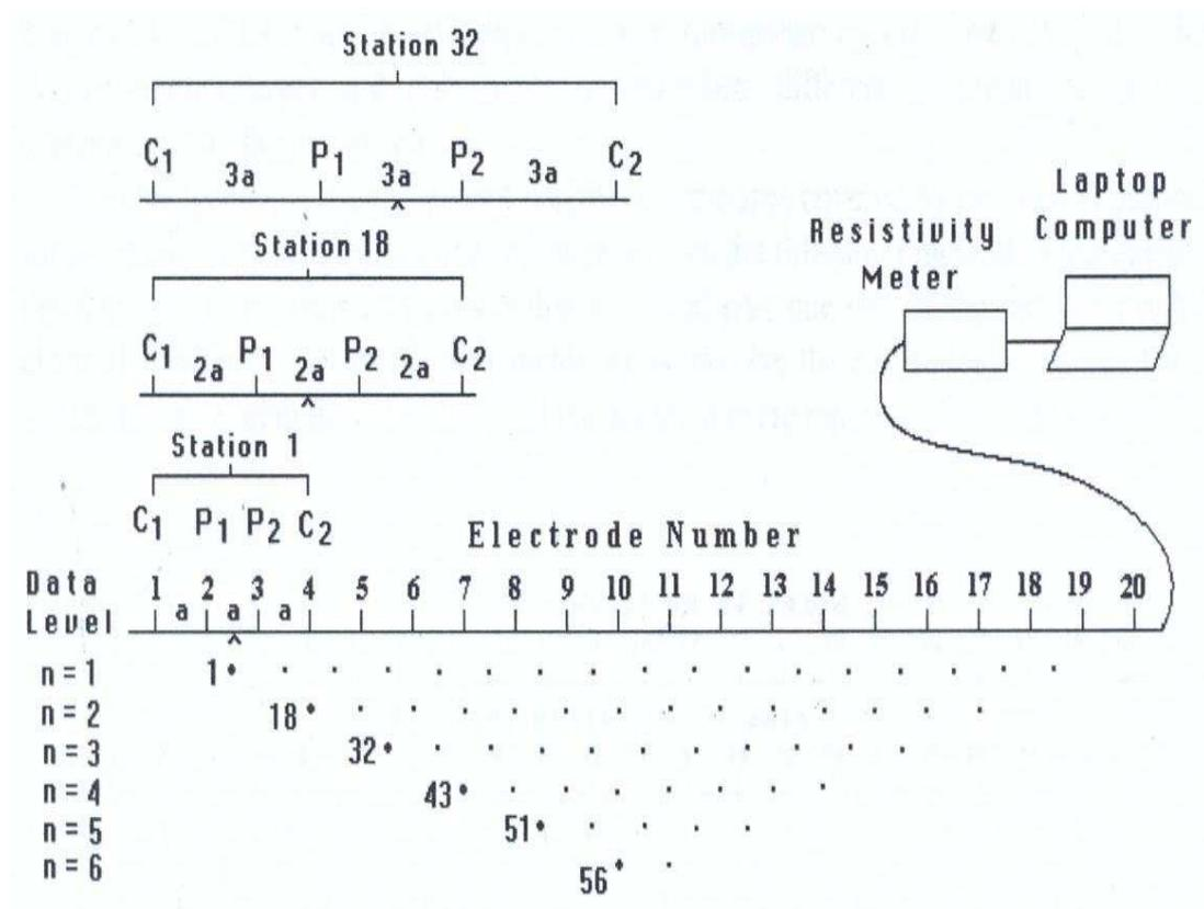
**Fig. 3.0:** The arrangement of electrodes for a 2-D electrical survey and the sequence of measurements used to build a pseudo section (Adapted from Loke, 1999).
