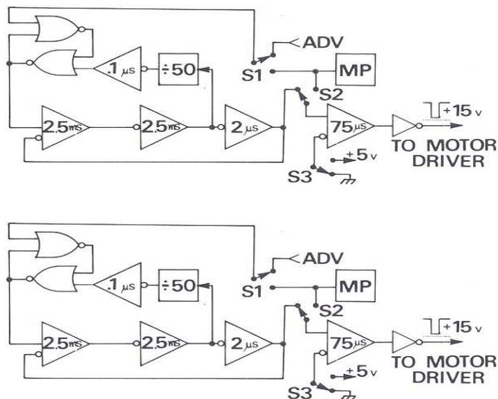
Fig.6-The simple pulse-train generator
