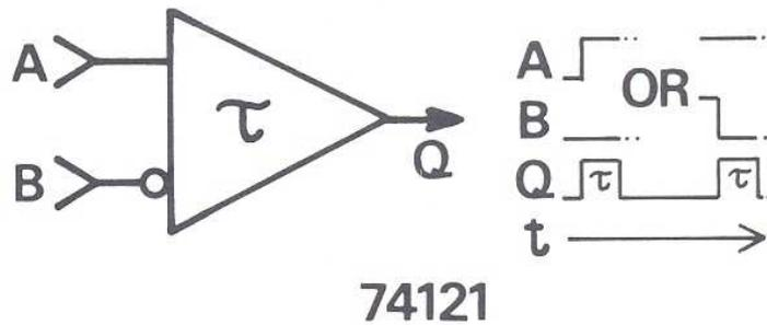
Fig.2-Operation of mono stable oscillator
