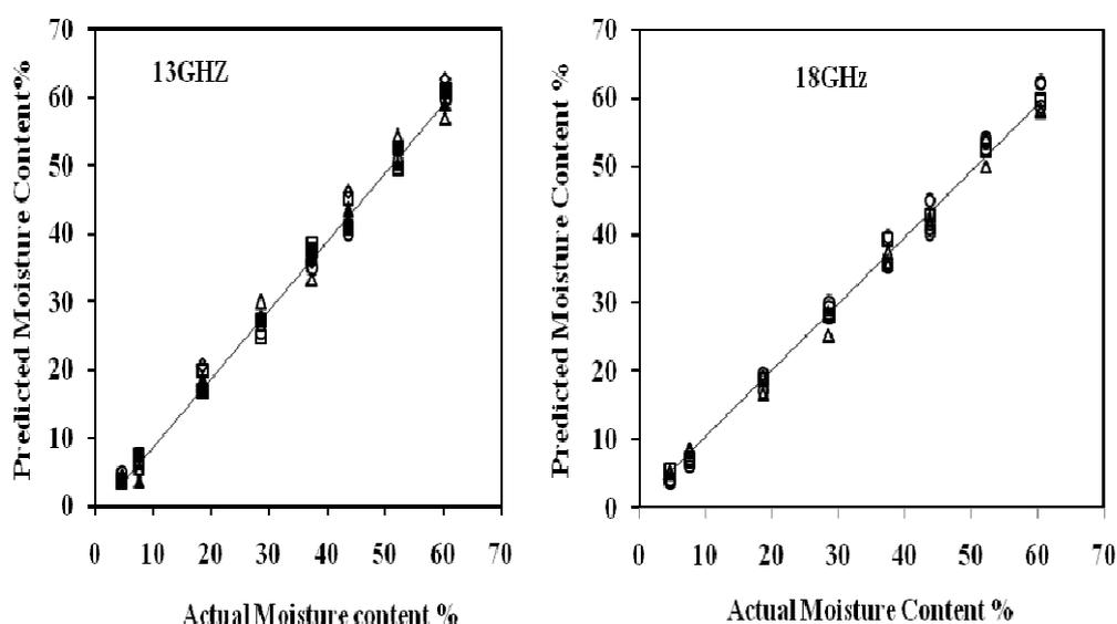
**Fig. 7 Predicted moisture content versus actual moisture content for soybean seed**
