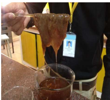
Fig. 4 Alginate fibres after bleaching
