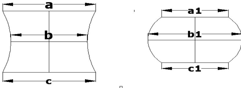
**Fig.5: Initial and final shapes of billet**
