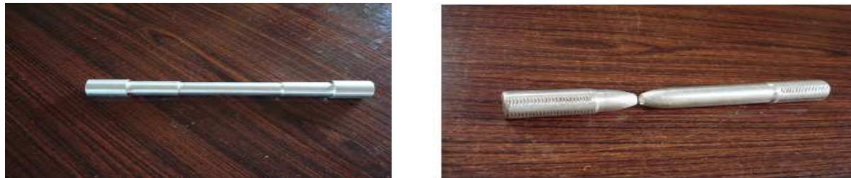
**Fig.6:** Tensile specimens (Before & after test)**Table.2: Material Properties**
