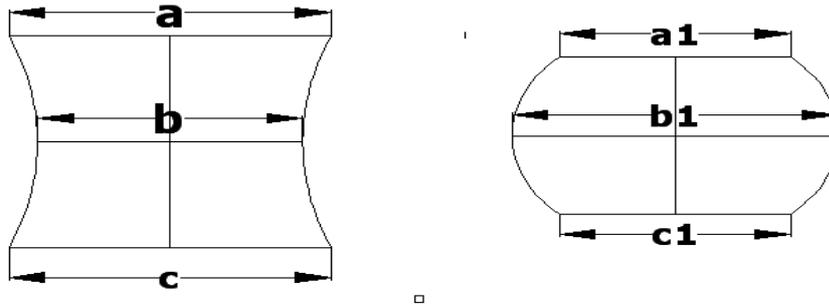
**Fig.5: Initial and final shapes of billet**
