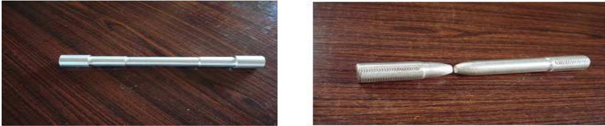
**Fig.6: Tensile specimens (Before & after test)**
