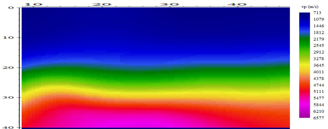
Figure 3: Seismic refraction tomography, showing the distribution of velocities within the subsurface
