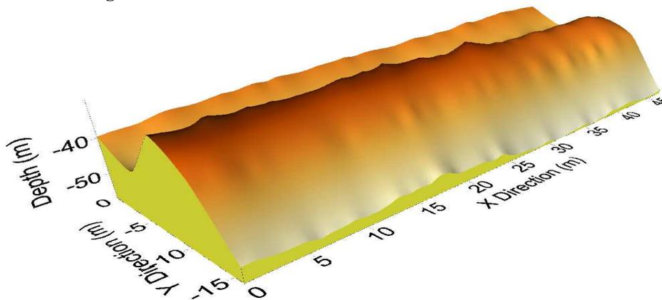
Figure 5: Generated 3D surface of the fresh basement
