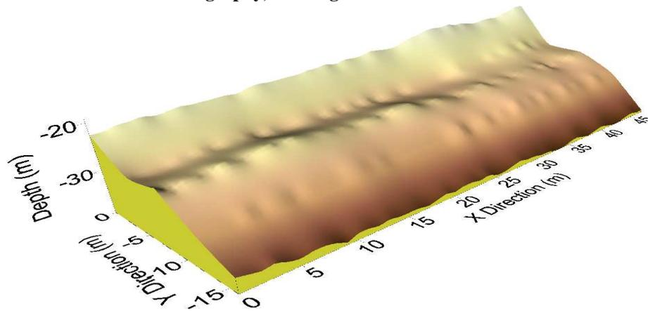
Figure 4: Generated 3D surface of the weathered basement
