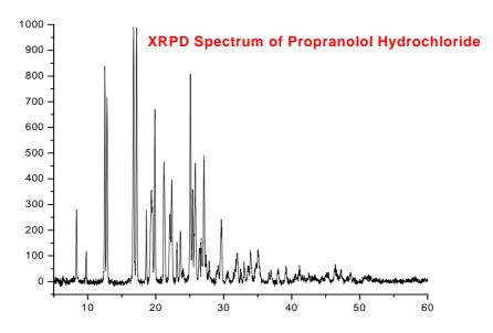
Fig. 6. XRPD spectrum of Propranolol hydrochloride
