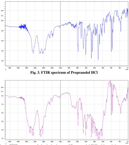
Fig. 4. FTIR spectrum of physical mixture of Propranolol HCl with excipients used
