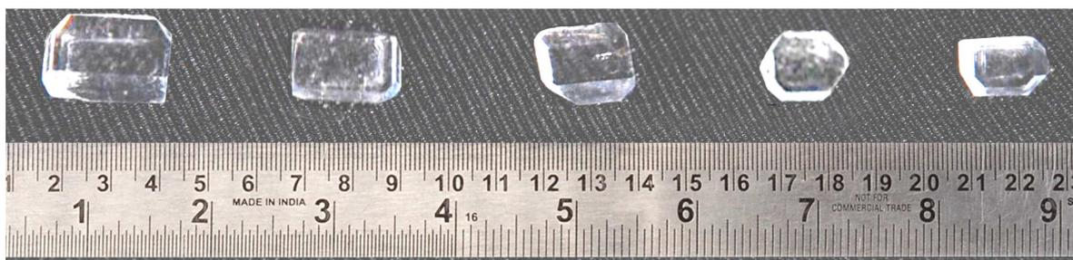
Figure 1: Photograph of the sample crystals grown From left are: Pure LAA, NaCl added LAA, KCl added LAA, glycine added LAA, and urea added LAA
