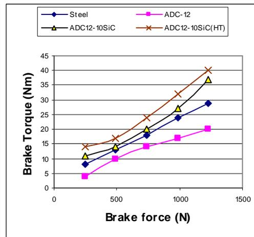
Fig. 6: Effect of brake force on brake torque at 60 km/hr
