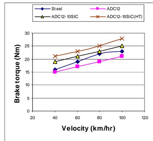
Fig. 12: Effect of velocity on brake torque at 984 N brake force
