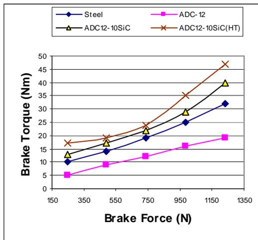
Fig. 7: Effect of brake force on brake torque at 80 km/hr
