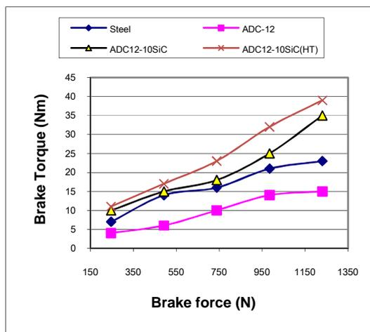
Fig. 5: Effect of brake force on brake torque at 40 km/hr
