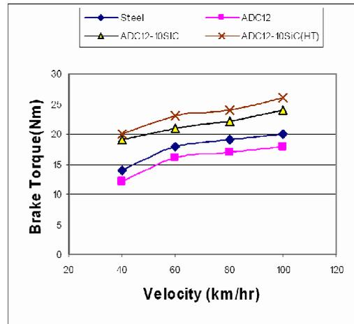
Fig. 10: Effect of velocity on brake torque at 492 N brake force
