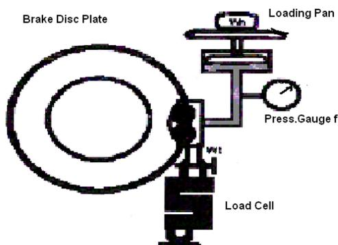
**Fig.3: Brake force application by weights through hand lever**
