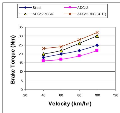
Fig. 13 :Effect of velocity on brake torque at 1230 N brake force
