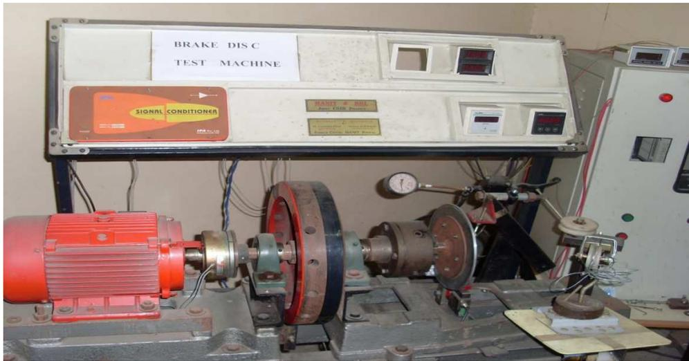
For selecting a suitable material for brake disc the simulation of brake disc operations is the best way to predict material suitability on the road. The test set-up has been designed for evaluating brake disc performance simulated operating conditions. Set up has been interfaced with computer with data acquisition facility to store data for subsequent systematic detailed analysis.
