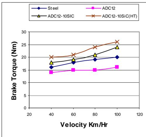
Fig. 11: Effect of velocity on brake torque at 738 N brake force
