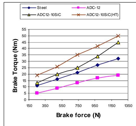
Fig.8: Effect of brake force on brake torque at 100 km/hr
