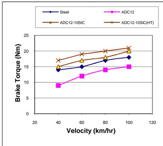
Fig. 9: Effect of velocity on brake torque at 246 N brake force
