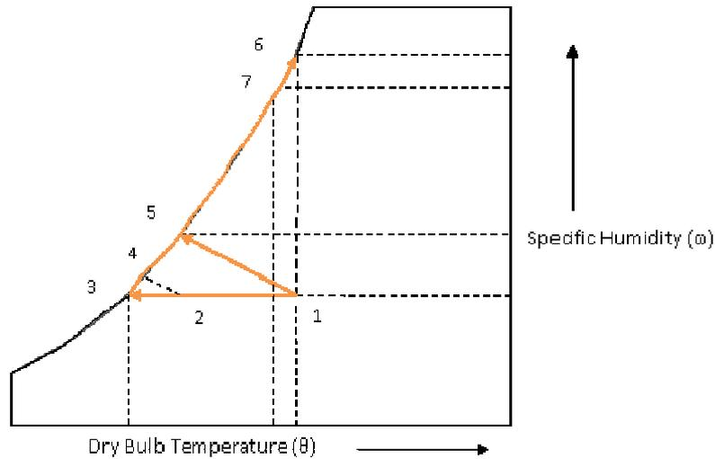
Fig. 2 Psychrometric Representation of working of a DPEC
