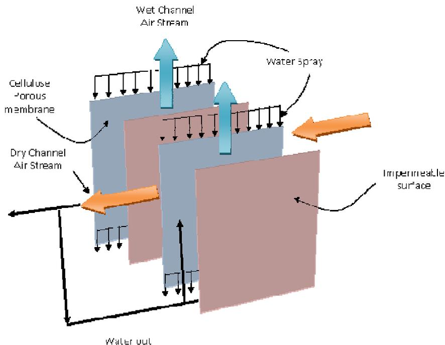
**Fig 1: Cellulose porous stack heat exchanger configuration of a novel DPEC**
