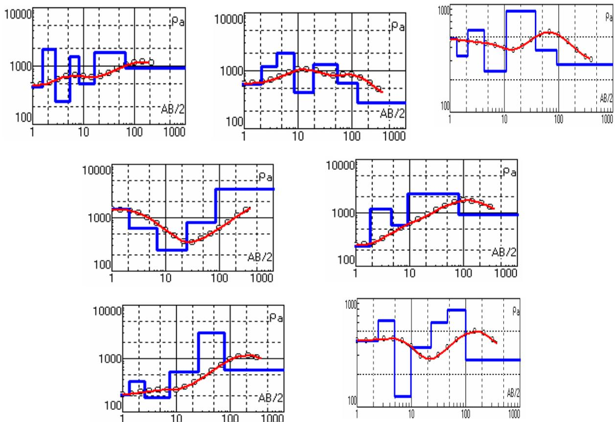
**Fig. 3: Interpreted Geoelectric model curves**
