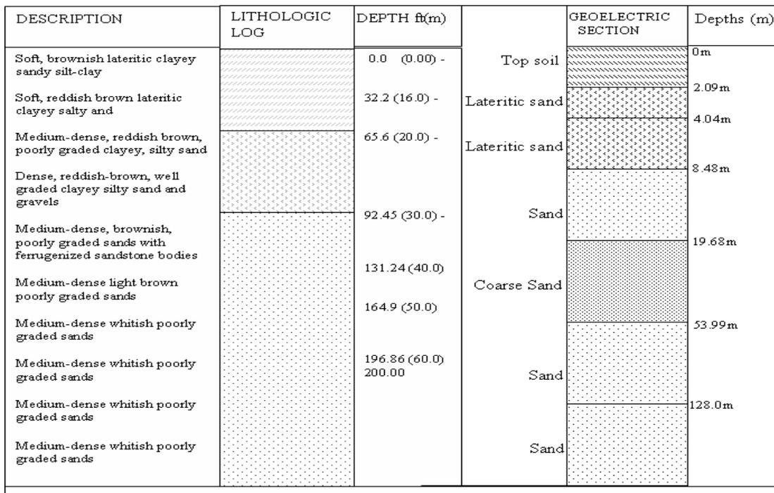
**Fig. 4: Lithologic Log and Interpreted Geoelectric sections**
