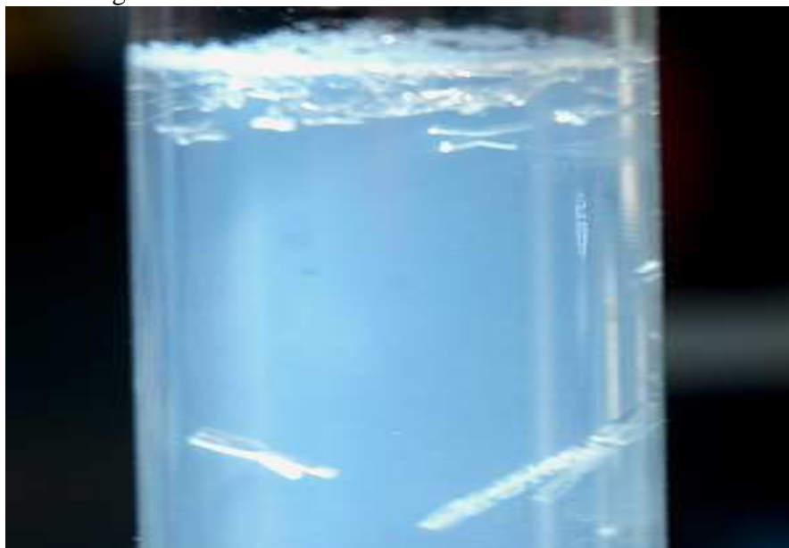
Fig. 1 Photograph of the grown \alpha - hopeite crystal
