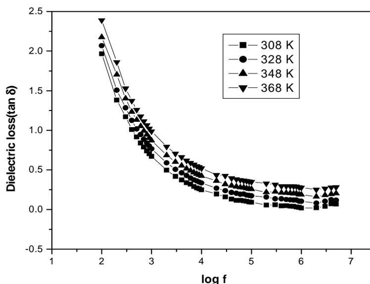
Fig. 6 Variation of dielectric loss with log frequency at different temperatures for LTN single crystal
