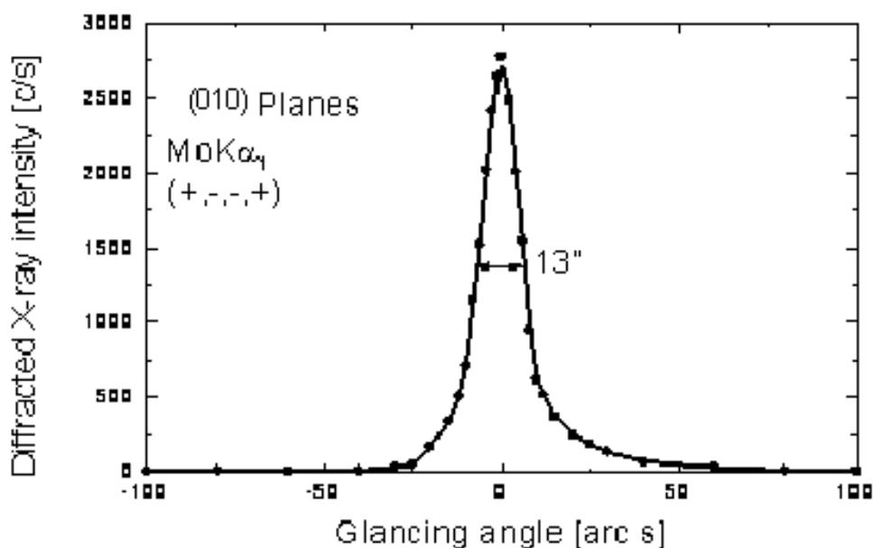
**Fig. 3 High-resolution diffraction curve recorded for LTN single crystal**
