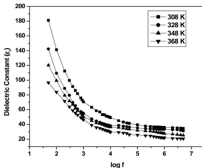
Fig.5 Variation of dielectric constant with log frequency at different temperatures for LTN single crystal
