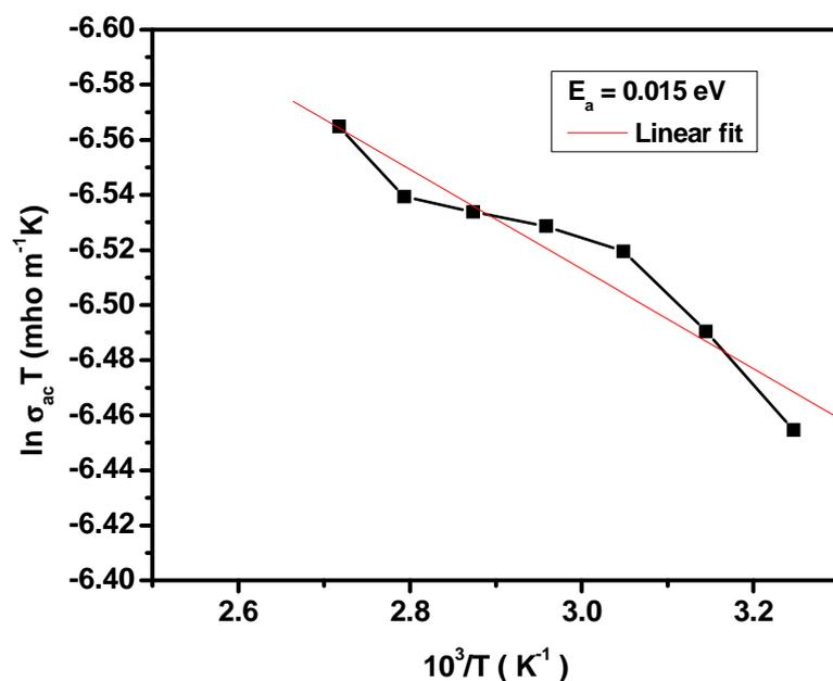
Fig. 8 Plot of  $\ln(\sigma_{ac})T$  versus  $1000/T$  for LTN
