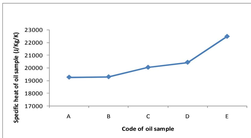
**Fig. 7:** A graph of comparison of specific heat capacities of oil samples A, B, C, D and E
