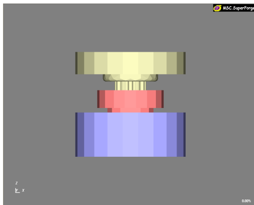
Fig.7: Assembled model die, punch and workpiece .
