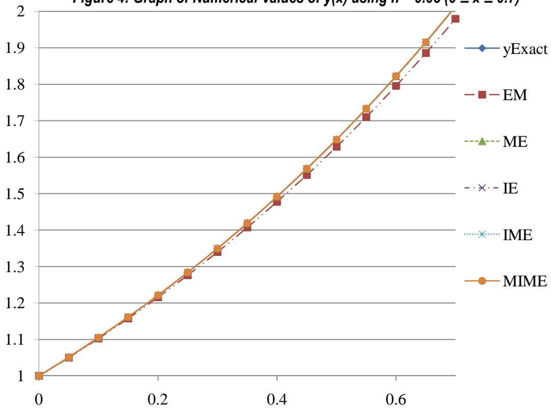
Figure 5: Graph of Numerical Values of  $y(x)$  using  $h = 0.5$  ( $0 \leq x \leq 0.7$ )
