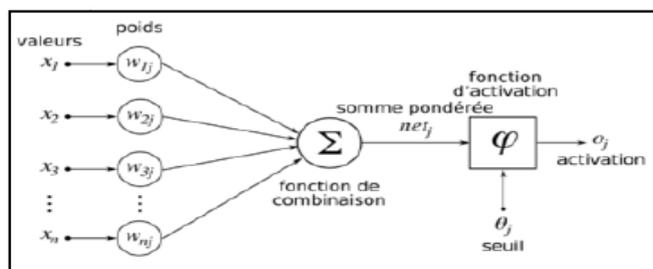
Figure 3: Structure of artificial neural
