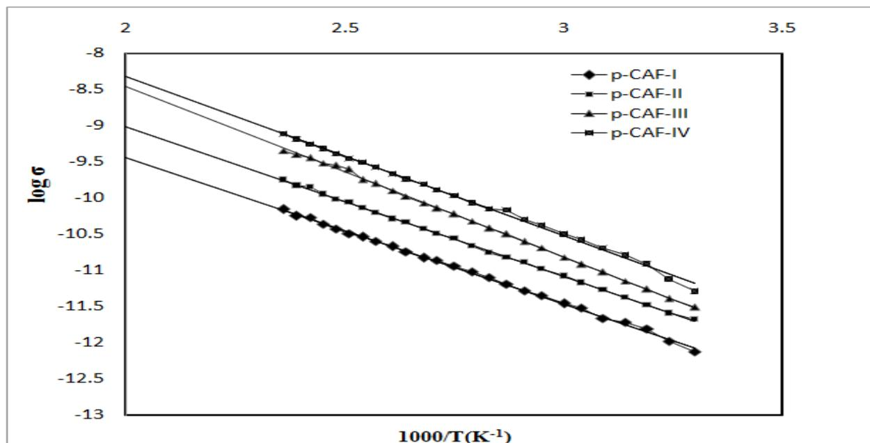
Figure 1: Electrical conductivity plots of p-CAF copolymers (Temperature dependence of  $\log \sigma$ )
