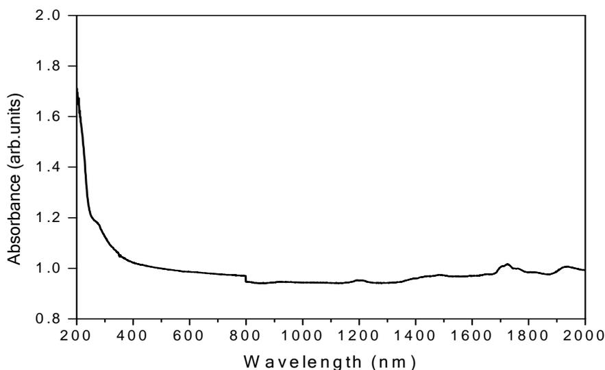
Figure 5 Optical absorption spectrum of LAO
