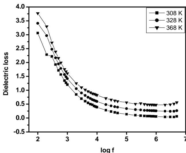
**Figure 8** Variation of dielectric loss with log frequency at different temperatures for LAO single crystal
