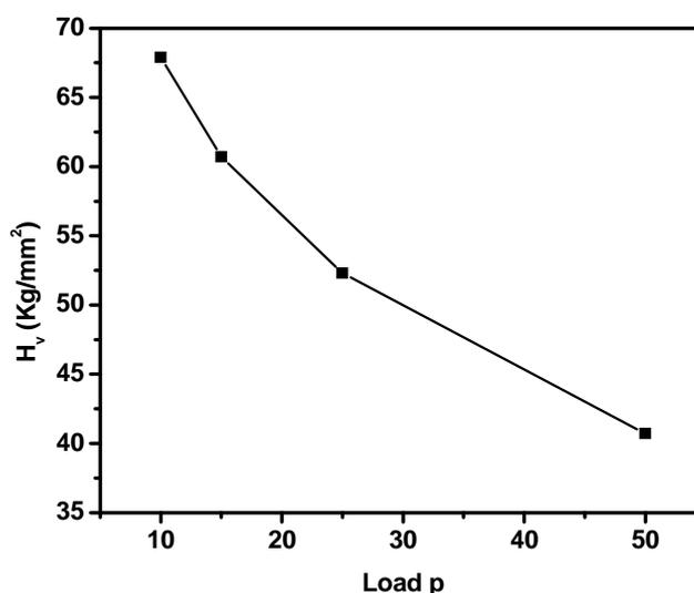
Figure 6 Variation of hardness with applied load for the plane (010)
