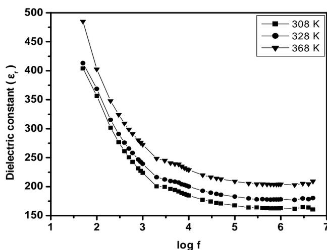
Figure 7 Variation of dielectric constant with log frequency at different temperatures for LAO single crystal
