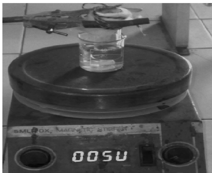
Figure 3 Modified disintegration test apparatus
