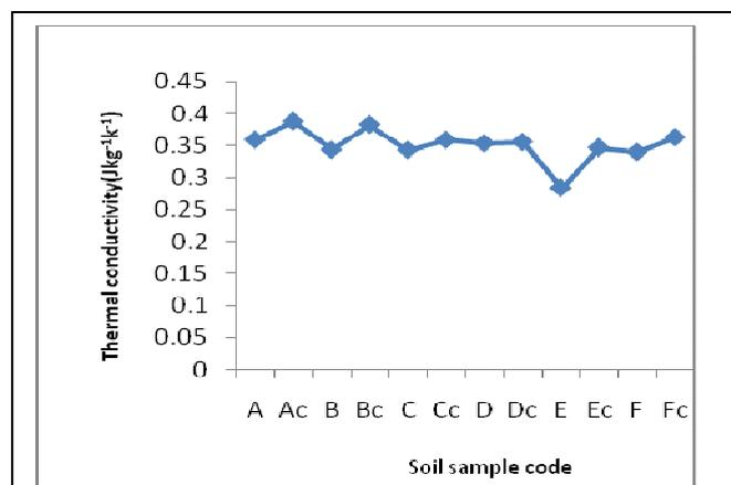
Fig.3: Variation of thermal conductivity with soil sample codes
