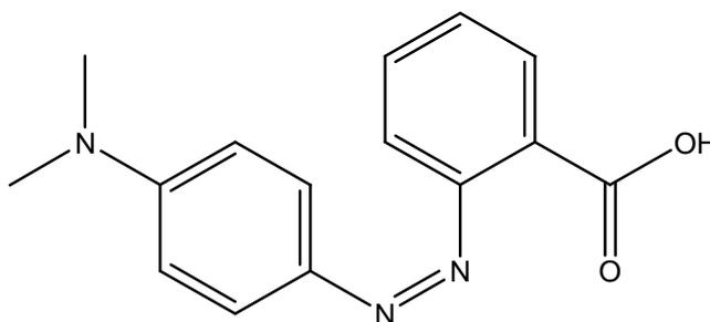
Figure 1: Molecular Structure of Methyl Red (MR)
