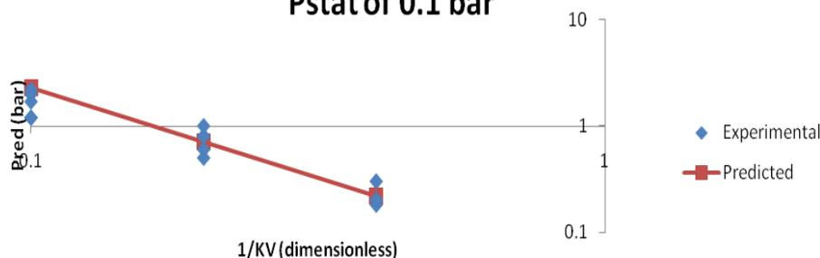
**Figure 2.0: Bartknecht Experimental results for methane-air**
