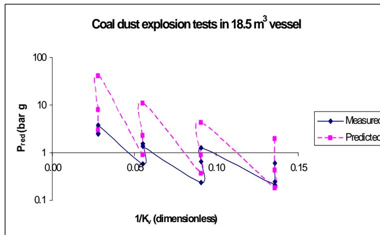
**Figure 3.3: Plot of measured and predicted peak pressures against  $1/K_v$**
