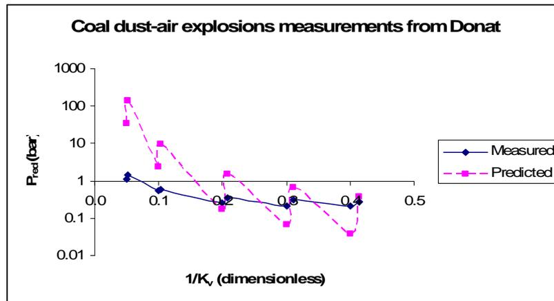
Figure 3.1: Plot of measured and predicted peak pressures against  $1/K_v$
