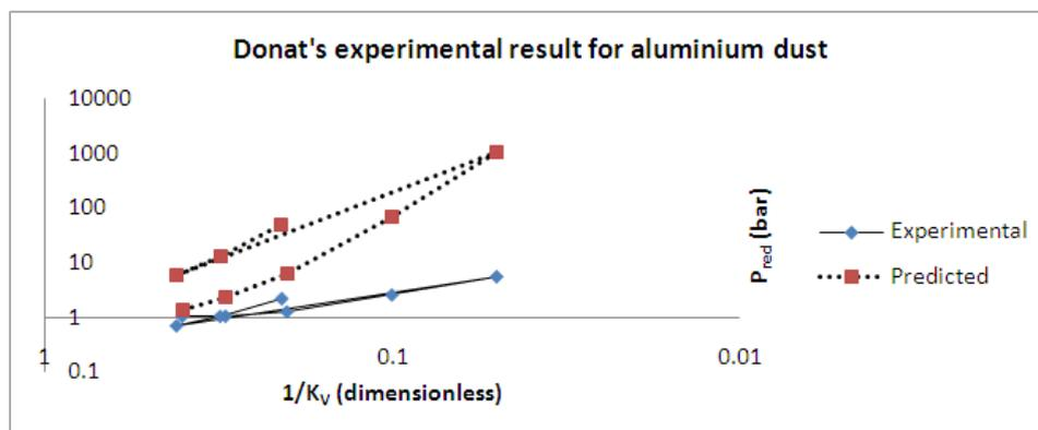
Fig 3.2: Plot of experimental and predicted  $P_{red}$  against  $1/k$
