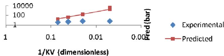
**Fig 2.5: Molkov experimental results and Bartknecht correlation Vs 1/K<sub>v</sub>.**
