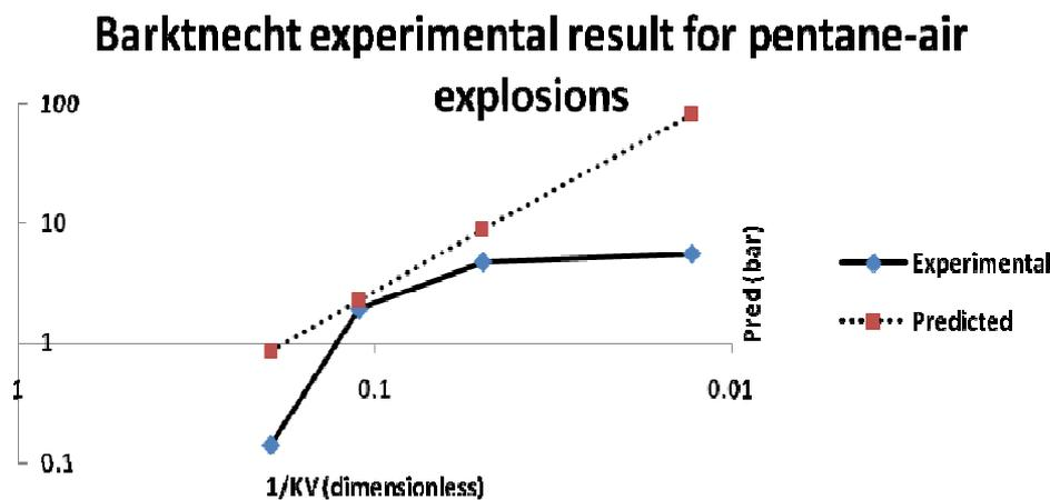
Figure 2.1: Graph of experimental result and predicted  $P_{red}$  versus  $1/K_v$
