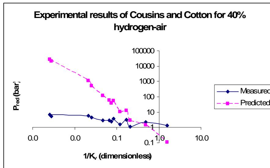
**Figure 2.2 Plot of measured and predicted peak pressures against  $1/K_v$**
