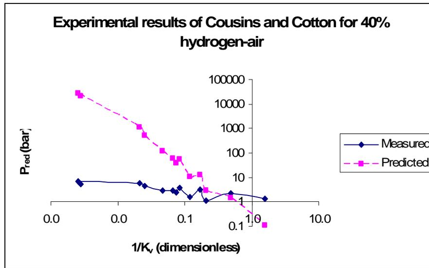
Figure 2.2 Plot of measured and predicted peak pressures against 1/ K<sub>v</sub>
