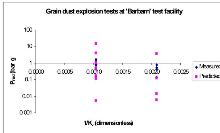
Figure 3.0: Plot of measured and predicted peak pressures against  $1/K_v$
