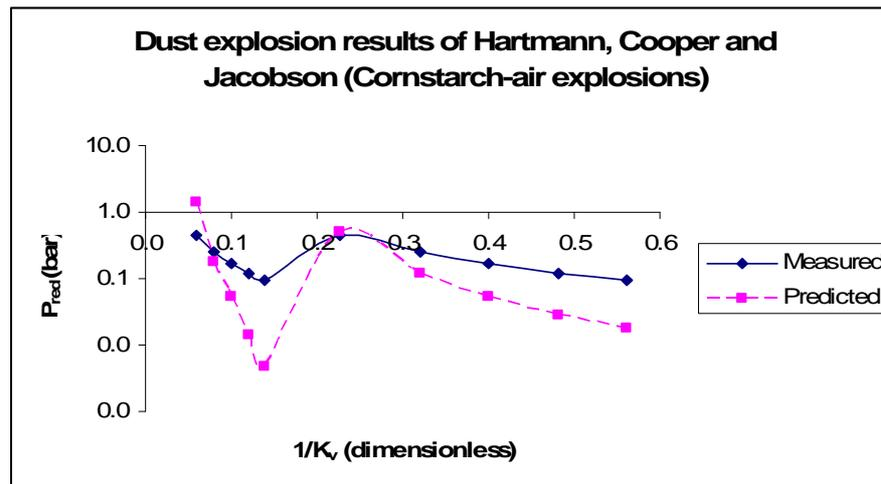
Figure 3.4: Plot of measured and predicted peak pressures against  $1/K_v$
