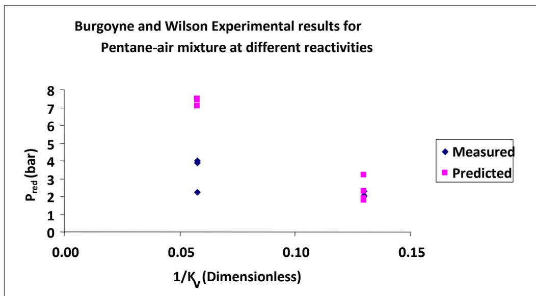
**Figure 2.4: Graph of measured and predicted peak pressures versus  $1/K_v$**
