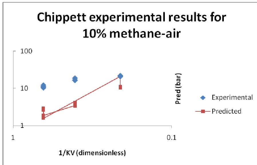
**Fig 2.3: Plot of experimental and predicted reduced maximum pressure against 1/K<sub>v</sub>**
