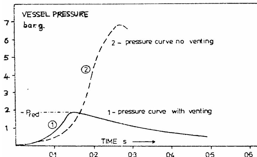
Figure 1.0: Explosion in a vessel with and without explosion vent for propane-air mixture
