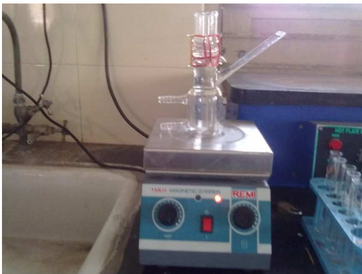
Fig 1: Modified Franz's diffusion cell for in vitro/ex vivo diffusion studies
