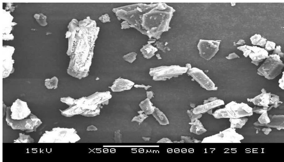
**Fig. 4:** Scanning electron microscope photograph of Rh6G
