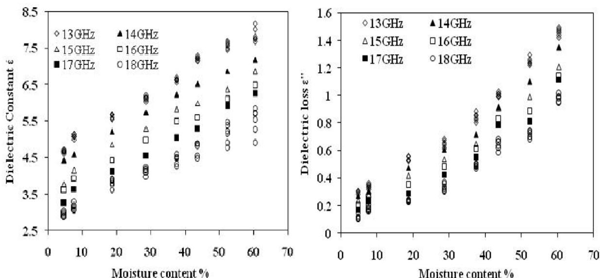
**Fig.4. Dielectric constant ( $\epsilon'$ ) and Dielectric Loss ( $\epsilon''$ ) as a function of moisture content (%) for Soybean seed at different frequencies**
