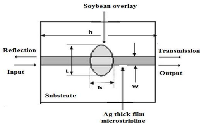
Fig.1: The schematic of Ag thick film microstripline with soybean overlay
