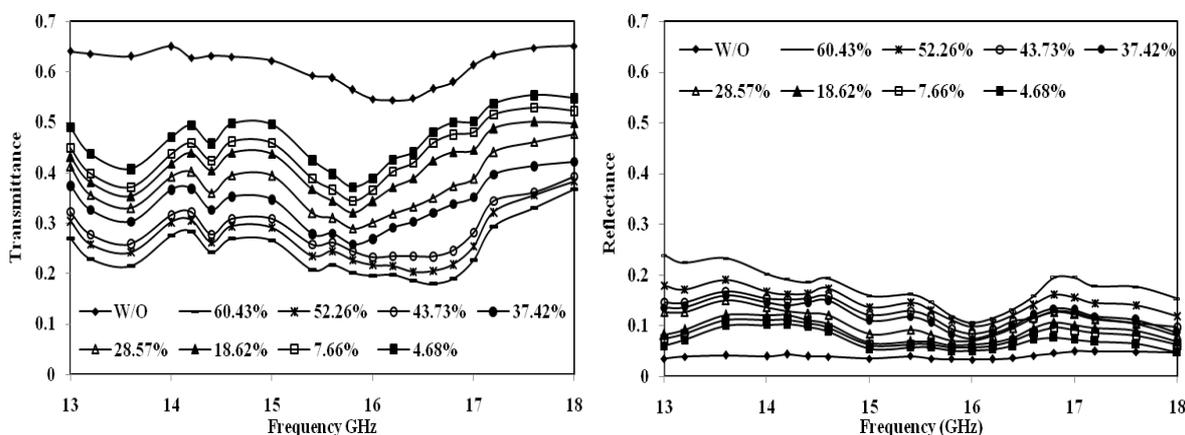
Fig.2. Perturbation in transmission and reflection due to seed overlay
