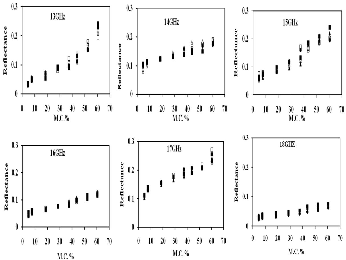
**Fig.3. Reflectance as a function of moisture content for various frequencies**
