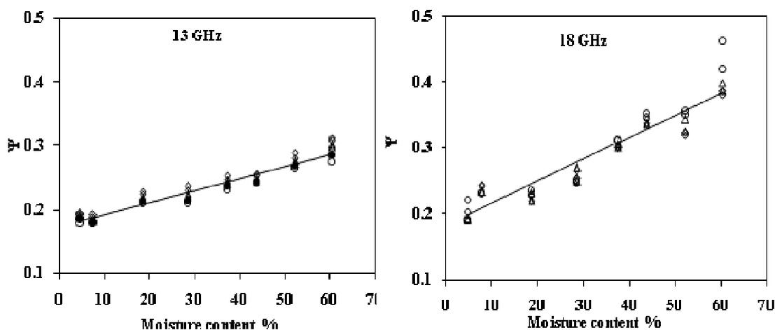
**Fig. 6 Moisture dependence of calibration function ( $\psi$ ) for soybean (six seeds)**
