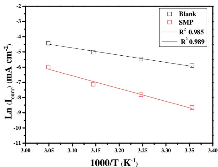
Figure 7. Arrhenius plots of carbon steel in 2.0 M  $H_3PO_4$  with and without  $5.10^{-4}$  M of SMP
