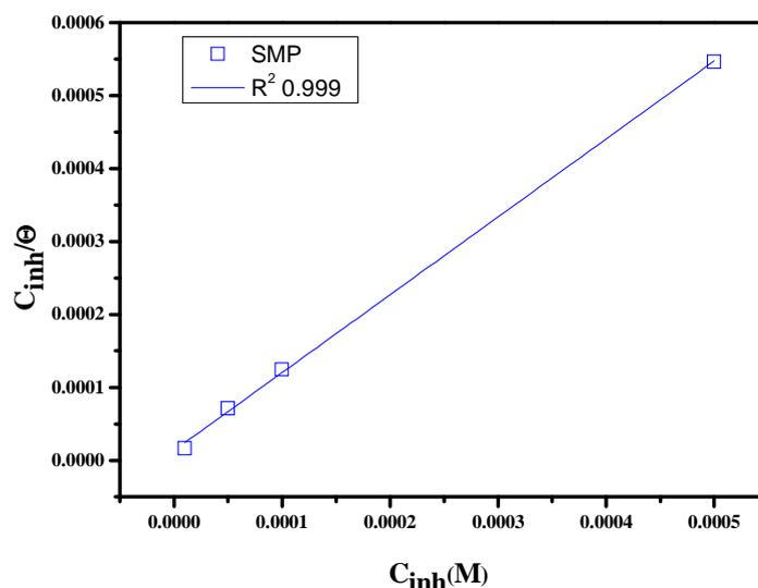
Figure 9. Adsorption isotherm according to Langmuir's model derived from EIS measurement
