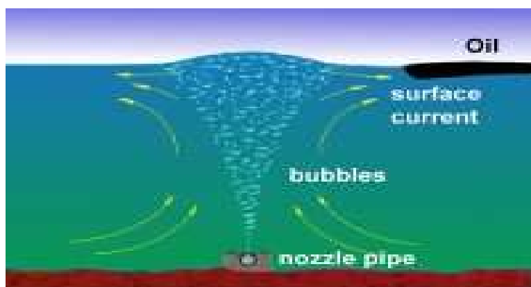
Figure 2 - Barriers (bubble) to prevent the spread of spilled oil on the water surface
