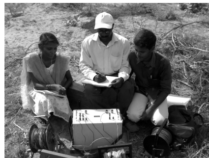
Figure.3. Square array electrical resistivity method data collection in the field
