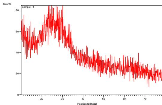
fig-3.1(d) XRD pattern of  $\text{Cd}_{0.6}\text{Te}_{0.2}\text{Se}_{0.2}$
