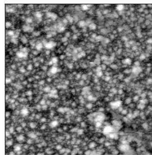
AFM pattern3.1(g)  $\text{CdSe}_{0.9}\text{Te}_{0.1}$
