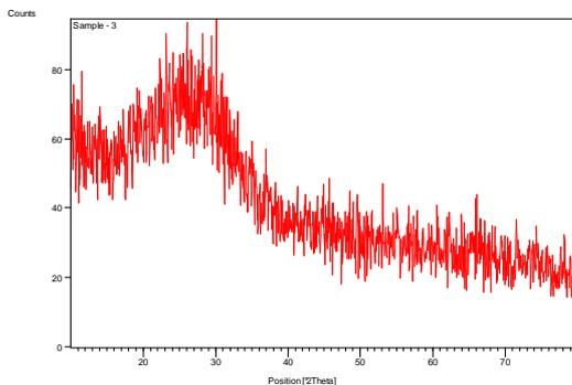
fig-3.1(c) XRD pattern of  $\text{Cd}_{0.7}\text{Te}_{0.2}\text{Se}_{0.1}$
