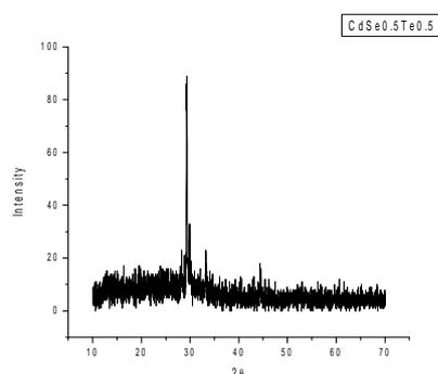
fig-3.1(b) XRD pattern of  $\text{CdTe}_{0.5}\text{Se}_{0.5}$
