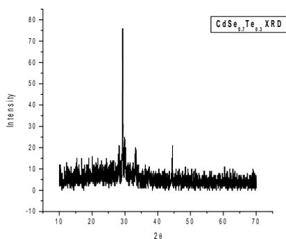
fig-3.1(a) XRD pattern of  $\text{CdTe}_{0.3}\text{Se}_{0.7}$
