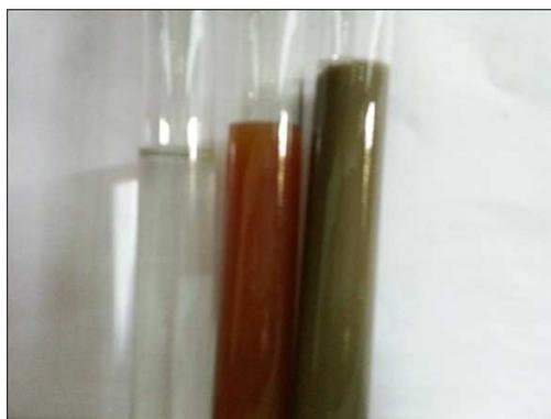
Figure 5: Showing colour changing. From left to right: 2mM AgNO<sub>3</sub>, *M. communis* Aqueous extract, Green synthesized silver nanoparticles aqueous product
