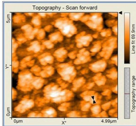
Fig. 4. Atomic Force Microscopis analysis of Silver nanoparticles
