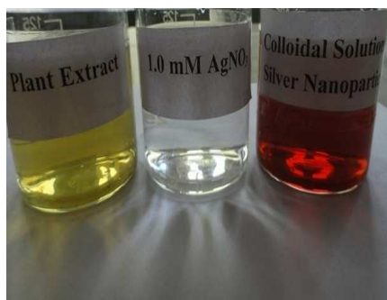
Fig. 1: Photograph of (A) Daturaalba Nees. leaf extract (B) 1.0 mM AgNO 3 solution without leaf extract (C) Colloidal solution of silver nanoparticles
