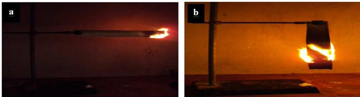
**Fig. 2 (a) Sandwich under horizontal Testing (b) Sandwich under vertical Testing**
