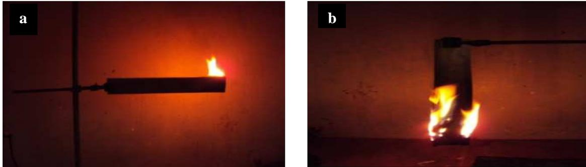
**Fig. 1 (a) PU foam core under horizontal Testing (b) PU foam core under vertical Testing**
