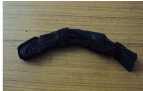
**Fig. 5 (b) Post burnt PU Foam (100 Kg/m<sup>3</sup>)**
