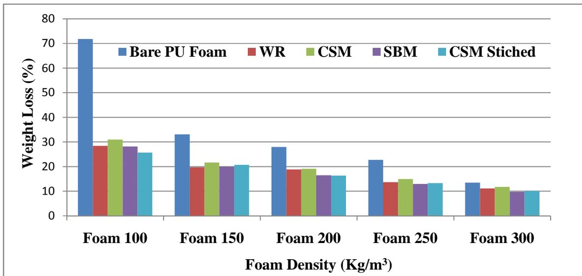
**Fig. 6 Loss of Weight (%) V/s foam density**
