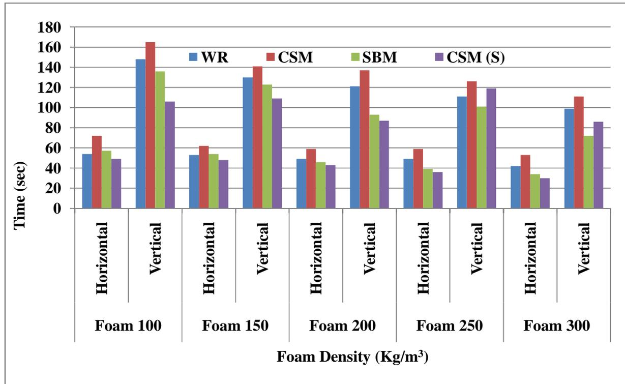
Fig. 3 Vertical and horizontal flame extinguishing time
