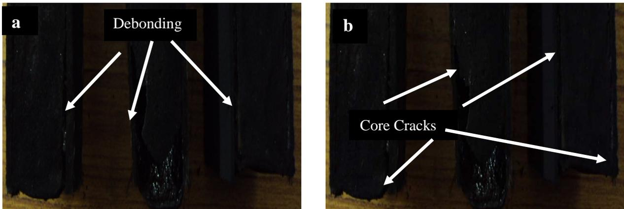
**Fig.7 (a) Face sheet debonding in sandwich composites 7 (b) core crack in sandwich composites**
