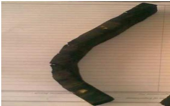
**Fig. 5 (a) Post burnt PU Foam (200 Kg/m<sup>3</sup>)**
