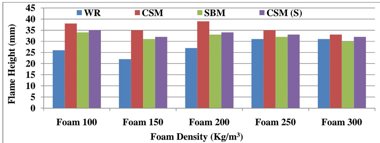
Fig. 4 Flame height V/s foam density in horizontal mode
