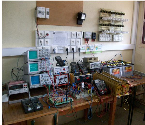
**Figure 3:** Measuring equipments set up to characterize the photovoltaic panels and systems.
