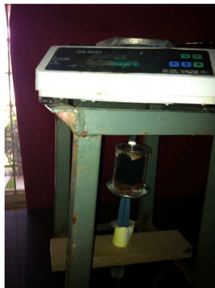
Fig 7: Modified electronic Balance with Hydraulic syringe system for measuring Mucoadhesive strength of tablets
