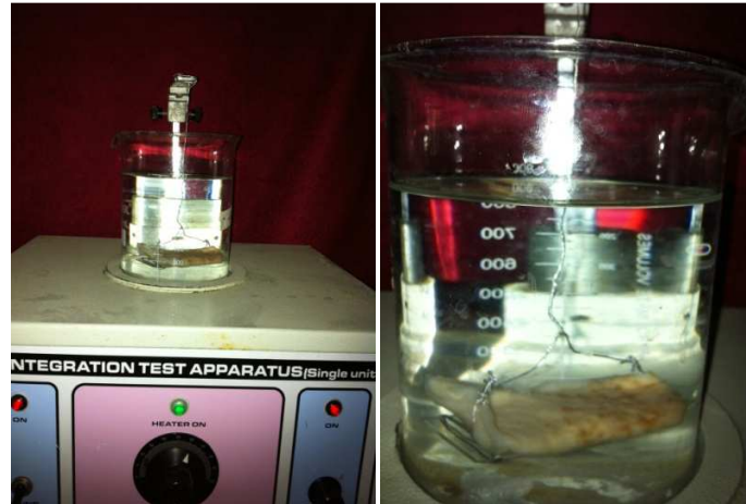
Fig 5 and 6: modified Disintegration Apparatus for Wash off Test
