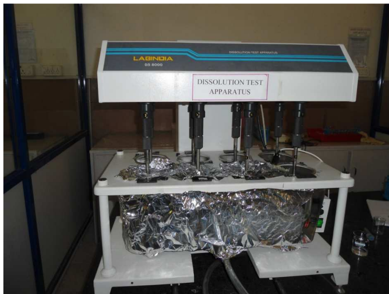
Fig 10 represents the LabIndia model USP type I dissolution apparatus covered with aluminium foil to prevent degradation of Montelukast sodium from light
