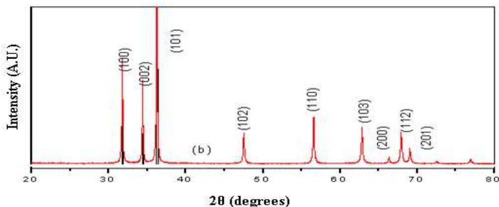
Fig.:1 X-ray Diffraction Pattern of ZnO Thick Film
