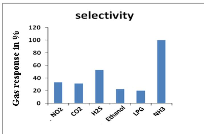
Fig. 5 Selectivity of ZnO sample for various gases
