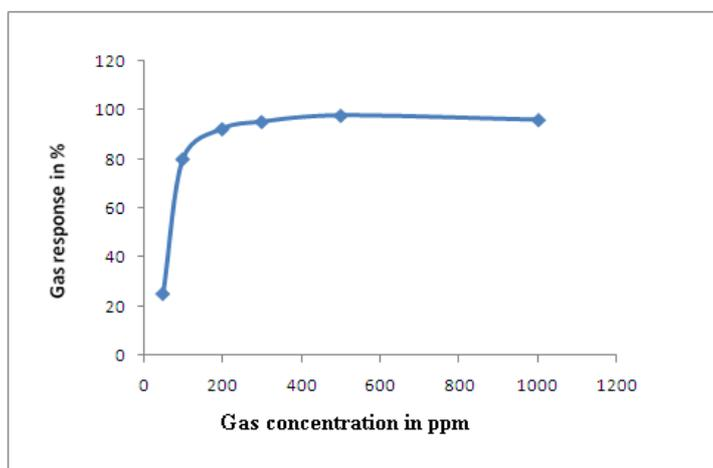
Fig.4. Variation of gas response with gas concentration
