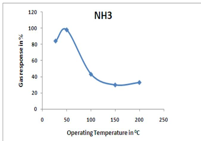
Fig.3. Variation of response with operating temperature for NH<sub>3</sub> gas at 500 ppm
