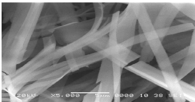
Fig.2: SEM micrograph of nano ZnO Thick Film
