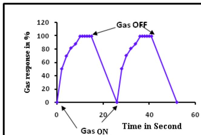
Fig. 6 Response and recovery of ZnO sample
