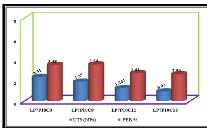
**Figure 1:** UTS and PEB values for LP7P10C0, LP7P10C9, LP7P10C12 and LP7P10C18 before and after degradation.
