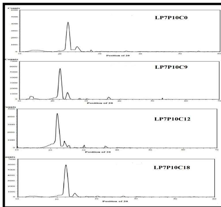
**Figure 2:** XRD patterns for LP7P10C0, LP7P10C9, LP7P10C12 and LP7P10C18 samples.
