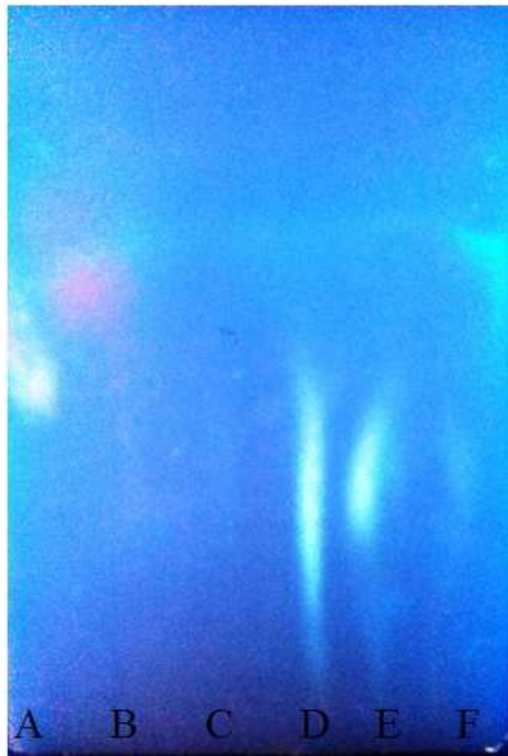
Fig. 2. Thin layer chromatography of (A) standard quercetin, (B) methanolic extract of ripe peel, (C) Methanolic extract of ripe pulp, (D) Ethanolic extract of ripe pulp and (E) Ethanolic extract of ripe peel of Musa acuminata
