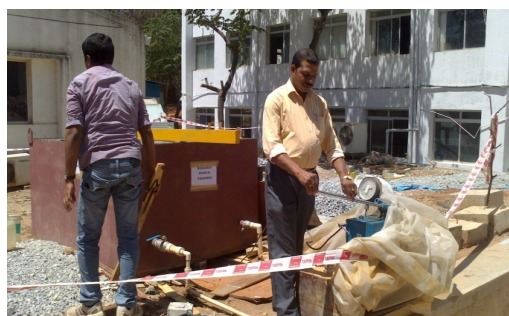
Figure 6: Gradient provision by Hydraulic Jack Arrangement to semi model pavement
