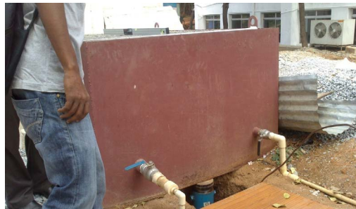
Figure 4: Rear Elevation of Fabricated Chamber showing Hydraulic Jack arrangement
