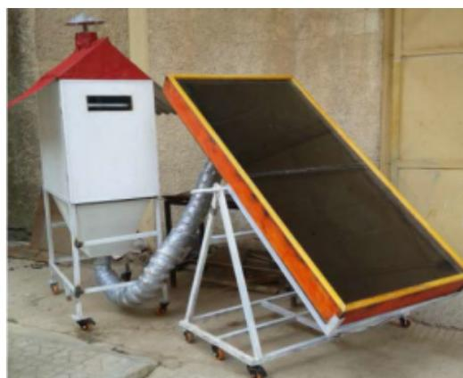
**Figure 2:** Photograph of solar forced convection dryer
