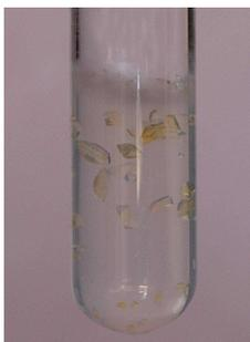
Fig. 1. Photograph of the grown SCBT single crystals
