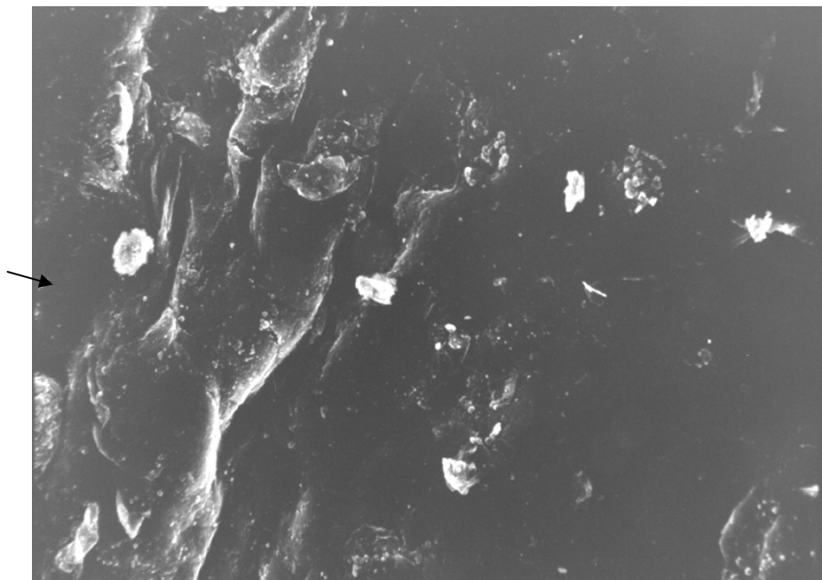
Figure 13: SEM photograph shows drug particles on the skin surface during their entry through skin appendage.
