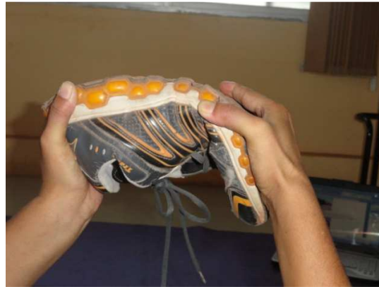
Figure 15 illustrate how sagittal stability of shoe was tested
