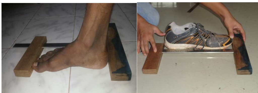
Figure 12&amp;13 illustrate how foot and shoe length evaluated
