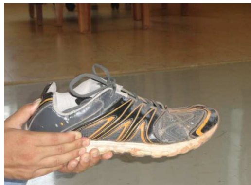
Figure 14 illustrate how heel counter stiffness evaluated
