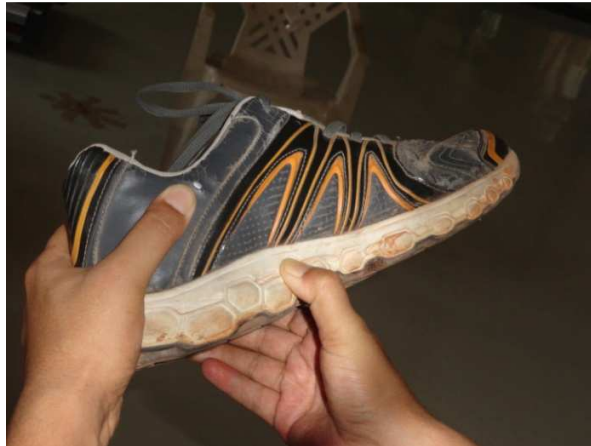
Figure 17 illustrate how lateral midsole hardness tested
