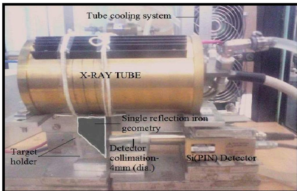
Fig. 2 Single reflection geometry set-up for photon irradiations
