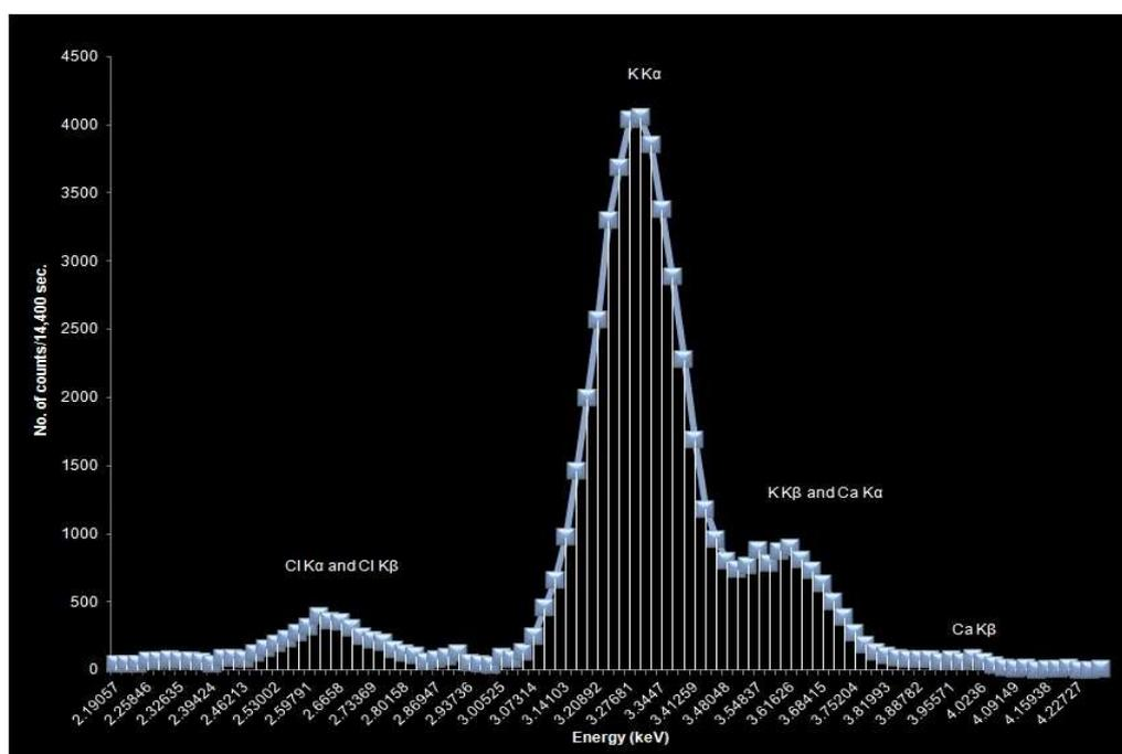
Fig. 3 Background subtracted spectrum of a maize sample irradiated with 5.959 keV photons from  $^{55}\text{Fe}$  source
