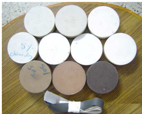
Photograph of virgin PTFE and its filled composite billets after sintering and skived tape
