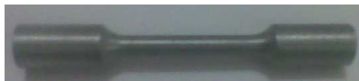
Fig: 2.6 - Test specimen of as cast Nickel Aluminium Bronze
