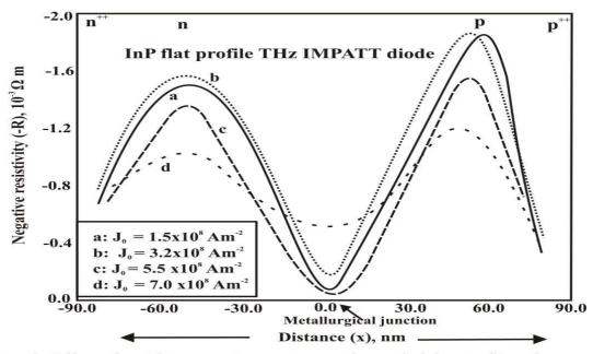
Figure 4. Effect of mobile space charge on negative resistivity profiles of InP Terahertz IMPATT diode at junction temperature = 250°C.
