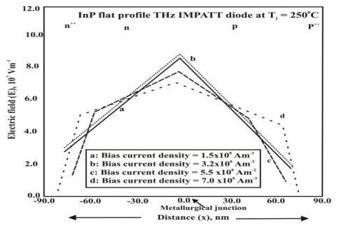
Figure 1. Effects of space charge on electric field profiles E(x) of InP DDR IMPATT diodes at elevated junction temperature
