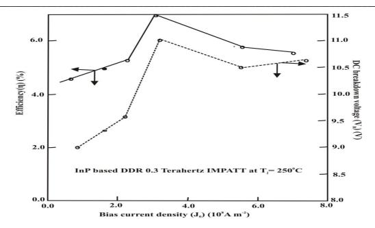
Figure 2. Effects of mobile space charge on Dc to RF conversion efficiency and breakdown voltage of the InP based 0.3 Terahertz IMPATT diode
