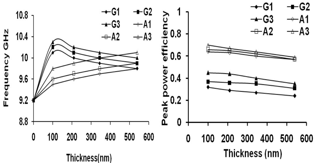
Fig.5. Resonance frequency and peak power efficiency as a function of thickness of Bi<sub>2</sub>O<sub>3</sub> thin film overlay (G1=A1=125°C, G2=A2=150°C and G3=A3=175°C)
