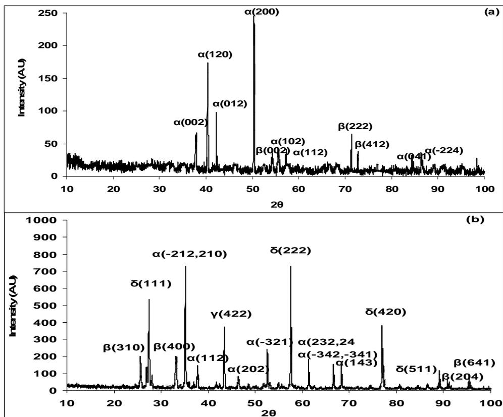
Fig. 1. XRD patterns of Bismuth oxide thin film on (a) glass (b) alumina
