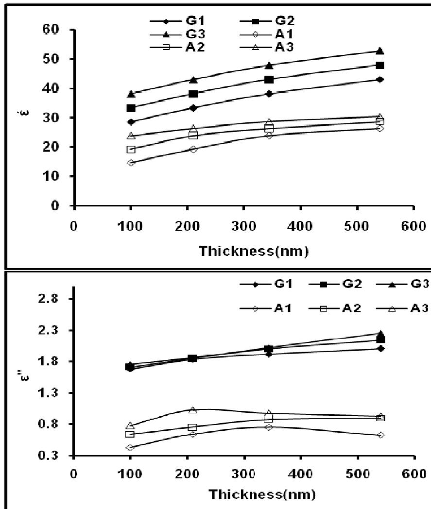
Fig.8. Permittivity of bismuth oxide thin film as a function of thickness
