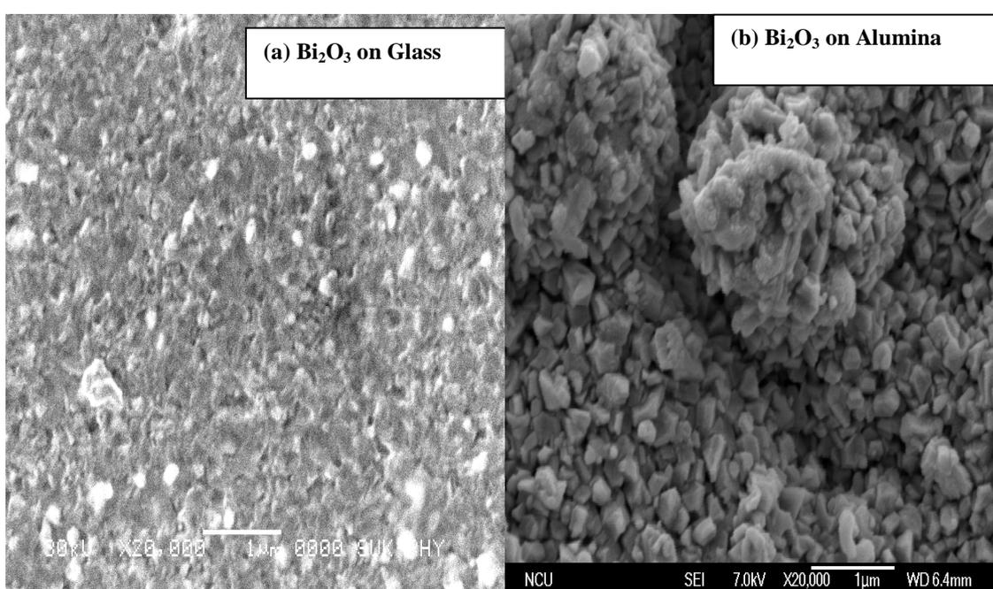
**Fig.2. SEM images of bismuth oxide thin film on (a) glass and (b) alumina for  $150^\circ\text{C}$
