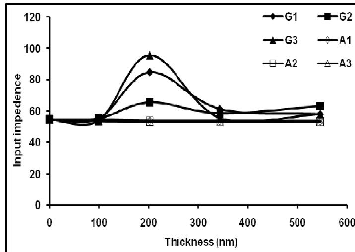
Fig.7. Input impedance of Ag thick film patch antenna as a function of thickness of overlay (G1=A1=125<sup>o</sup>C, G2=A2=150<sup>o</sup>C and G3=A3=175<sup>o</sup>C)
