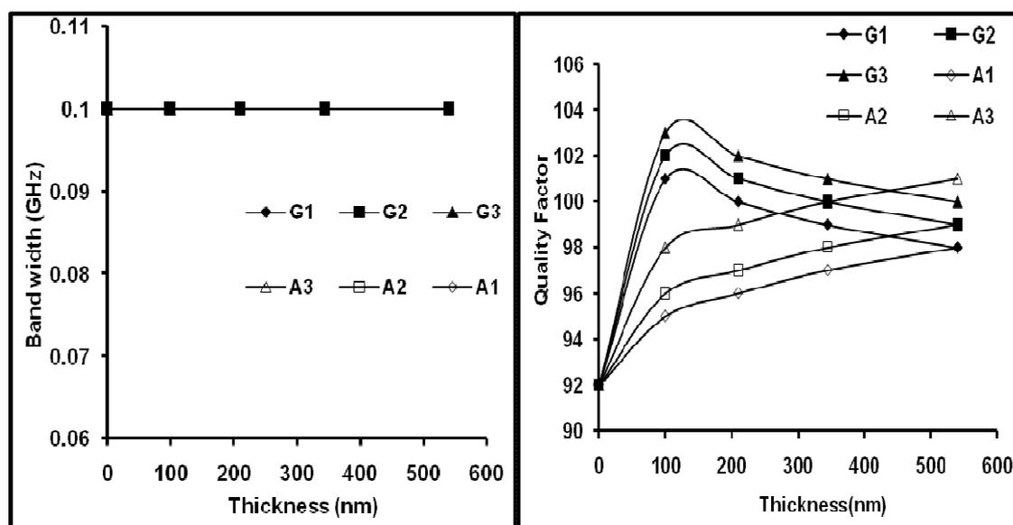
Fig.6. Bandwidth and Quality factor of antenna due to bismuth oxide thin films overlay as a function of thickness (G1=A1=125<sup>o</sup>C, G2=A2=150<sup>o</sup>C and G3=A3=175<sup>o</sup>)
