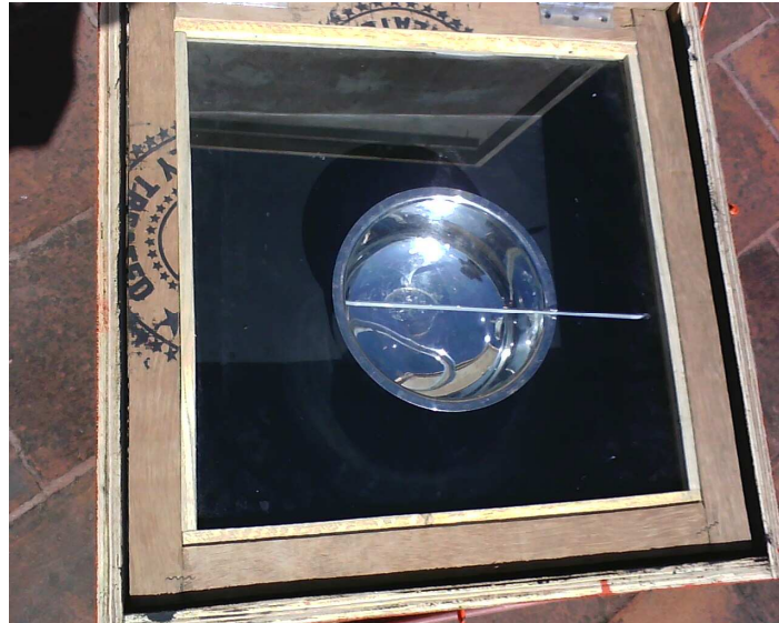
Fig. 11 Solar cooker with a stainless steel vessel for temperature profiling
