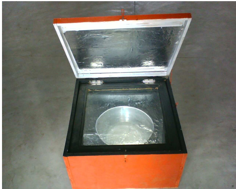
Fig. 14: Solar Cooker with concentrator (view 1)
